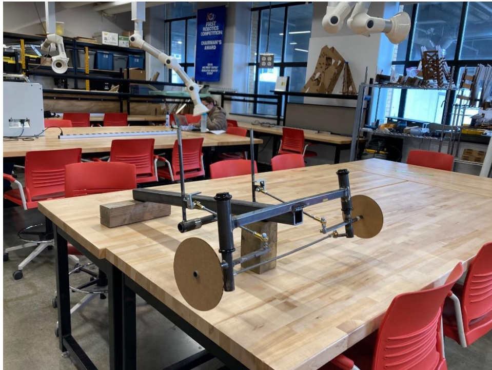
Figure 7.6: Final result of prototype, cardboard wheels laser cut for demonstration and steering stops added to prevent linkage from going in reverse.
