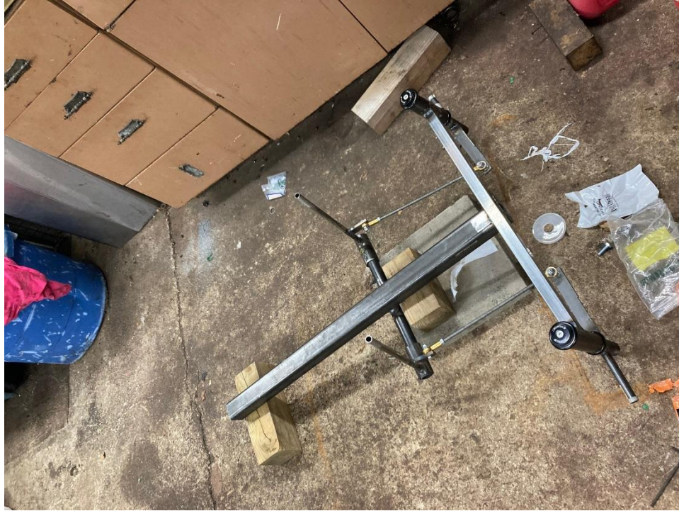
Figure 7.5: Threaded rods cut to length and prototype fully assembled and bolted together
