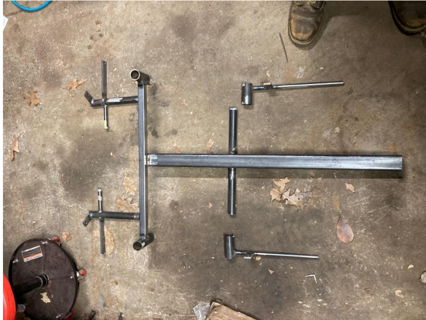
Figure 7.3: All pieces welded together into sub-assemblies
