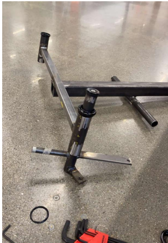
Figure 7.4: Headset bearings pressed into headsets
